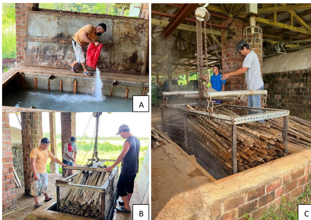
Figure 1. The treatment process of laminated bamboo slats using a borax and boric acid solution. (A) Preparation of the treatment solution by dissolving borax and boric acid in heated water within the treatment tub. (B) Gradual submersion of bamboo slats into the solution using a pulley system. (C) Retrieval of bamboo slats after 72 hours of immersion in the heated treatment solution.
