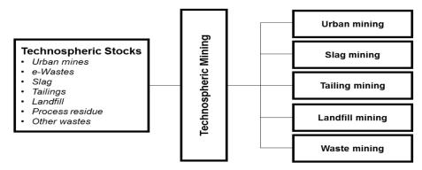
Figure 1. General concept of technospheric mining (adapted from N. Johansson et al., 2013).
