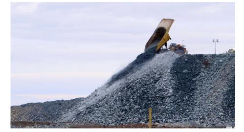
Figure 2. Mine wastes are technospheric stocks and can be utilized for metal or mineral resource recovery as part of technospheric mining (photo: https://research.curtin.edu.au/industry-partners/invest/resources/mine-waste-management/)
