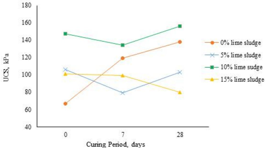
Figure 5. Effect of Curing Period on the UCS
