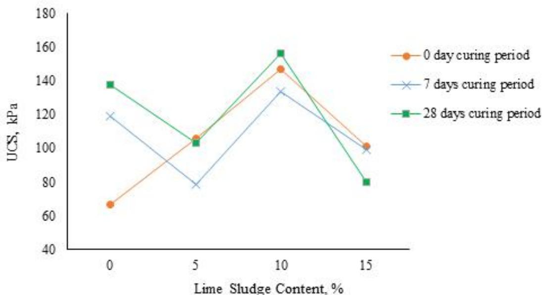
Figure 4. Effect of Sugar Mill Lime Sludge on the UCS
