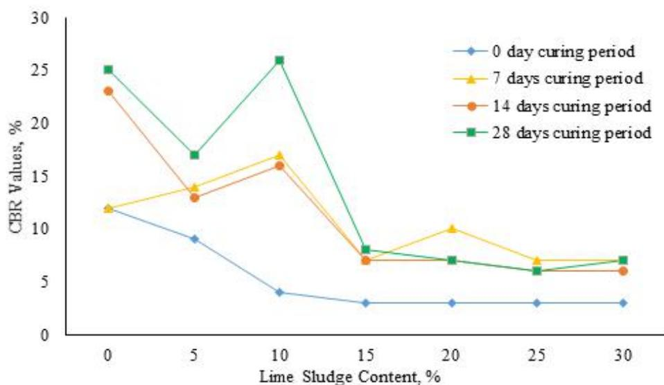
Figure 2. Effect of Sugar Mill Lime Sludge on the CBR
