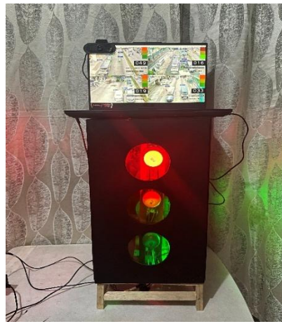
Figure 10. A prototype of Internet of Things-based traffic light control showing output based on video feed
