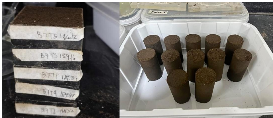
Figure 3. Prepared specimens being cured for direct shear and triaxial test.
