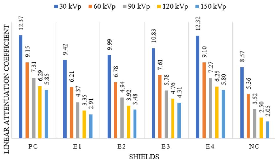
Figure 1. Linear attenuation coefficient (measured in cm<sup>-1</sup>) of shields
