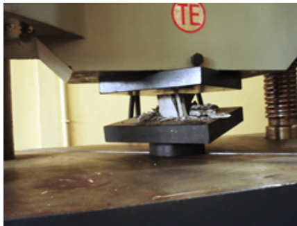
b) Mortar specimen at failure
