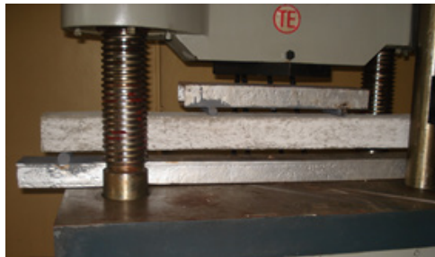
Figure 3. The Typical Set-Up of the Third-Point Load Tests Using the UTM
