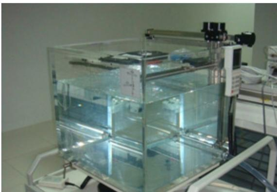
**Figure 6.** Water phantom and its scanning system.
